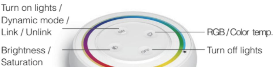
Touch ring: brightness, saturation, color temperature, RGB use together.
